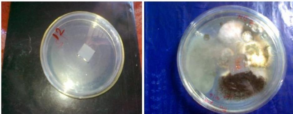
**Figure 8:** Evidence of fungi growth (*A.Niger*) on surface of LDPE films with and without low molecular weight chitosan.
