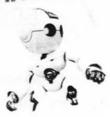
the alpha humanoid robot has a body articulated via 16 servo motor like joints with their corresponding muscles. That's give it a superb range of movements. It can dance walk and do kung-tu.
