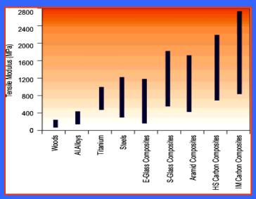
The lowest properties for each material are associated with simple manufacturing processes and material forms (e.g. spray lay-up glass fibre), and the higher properties are associated with higher technology manufacture (e.g. autoclave moulding of unidirectional glass fibre), the aerospace industry.
