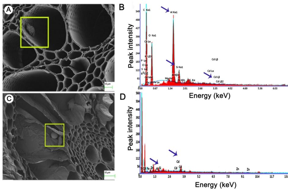
Fig.1. SEM image and EDX spectrums of the electron dense depositions in the root vessel of maize and rice exposed to CdCl<sub>2</sub> stress.
